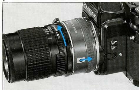
1. Remove the lens from the camera. Attach it to the camera body in the similar way as the lens is attached to the body.
