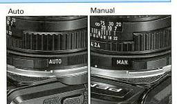
To preview the depth of field or to operate the diaphragm manually, slide the lever downward as shown in the photo. The lever will lock on manual (MAN.). To reengage the automatic diaphragm, press the lever. The lever will spring back to the AUTO position.
